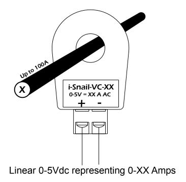
i-Snail devices must be installed on INSULATED conductors only.
