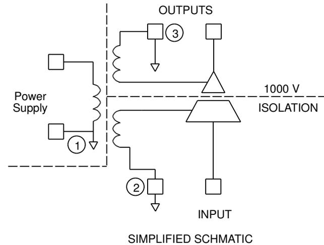
Power Supply, Input and Output are all isolated;
