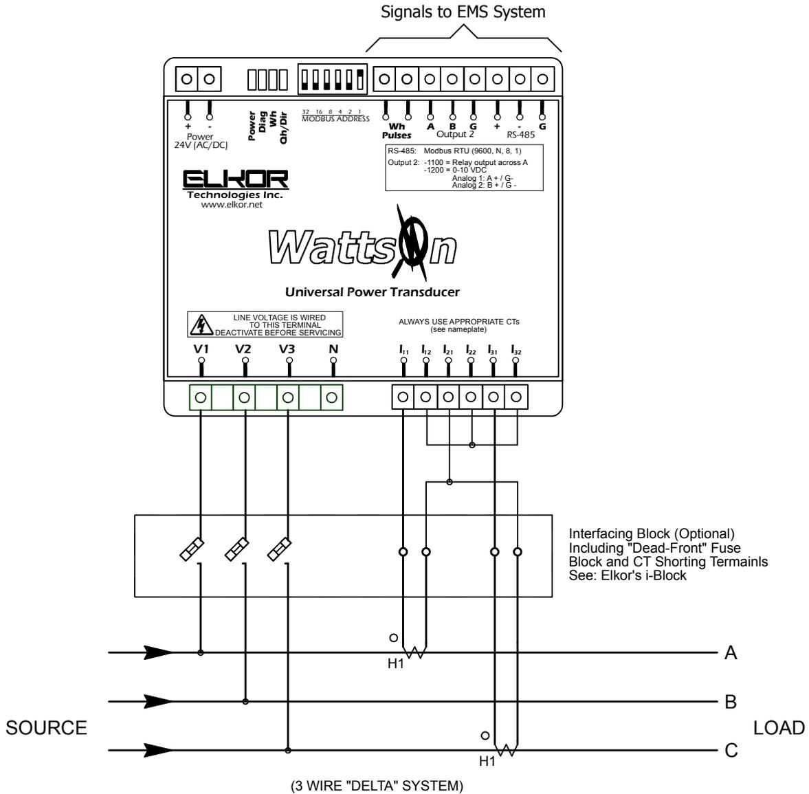
**WARNING: This wiring method works only with 5A meters/CTs. When using mV or mA CTs, the 3 wire, 3 CT method must be used as per Appending 1B.**
