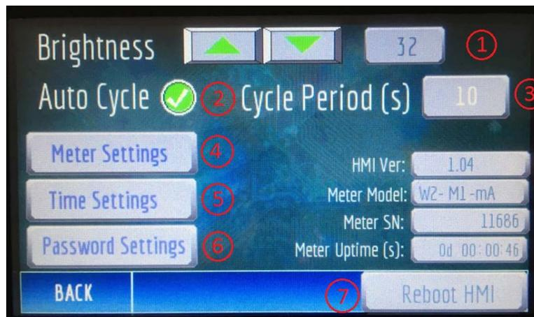
The "Meter Uptime" and "Meter SN" fields are useful to diagnose proper communication between the LCD and the meter as they are polled from the meter by the LCD.
