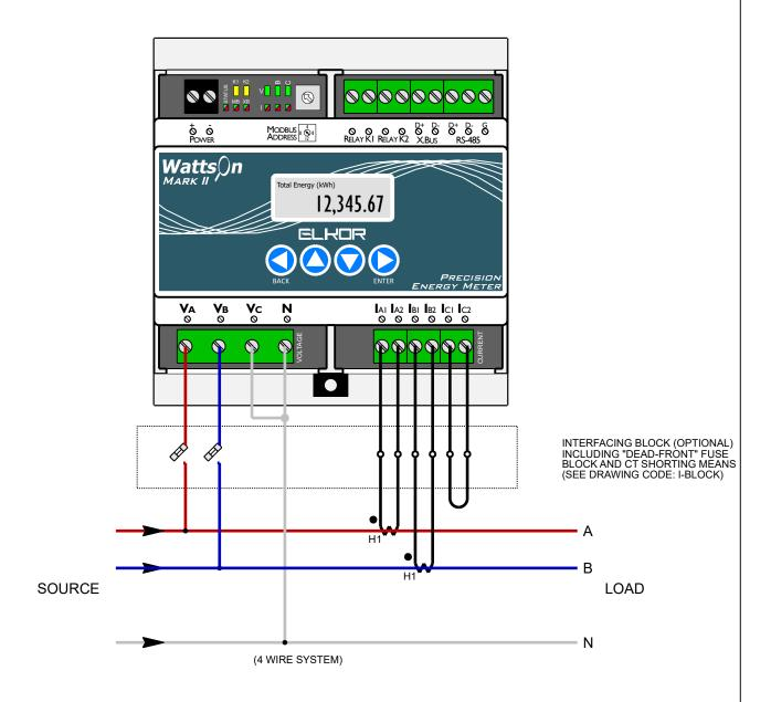
WIRING USING STANDARD 5A CTs SHOWN. WHEN USING 5A CTs, ELKOR RECOMMENDS THE USE OF A SHORTING BLOCK.
