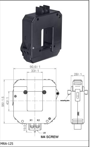
Unlike standard 5A CTs, MRA Current Transformers do not produce high voltages when opened. They generate a low energy mA signal level and no special protection and/or shorting blocks are required. Maximum open secondary voltage is clamped at about 7V ac.
